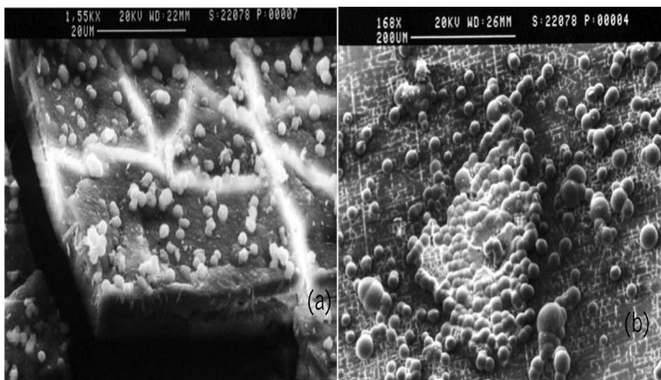
FIGURE 8. SEM micrograph of (a) gallium doped (b) Indium doped glass sample soaked in SBF for 7 days.<sup>134</sup>
