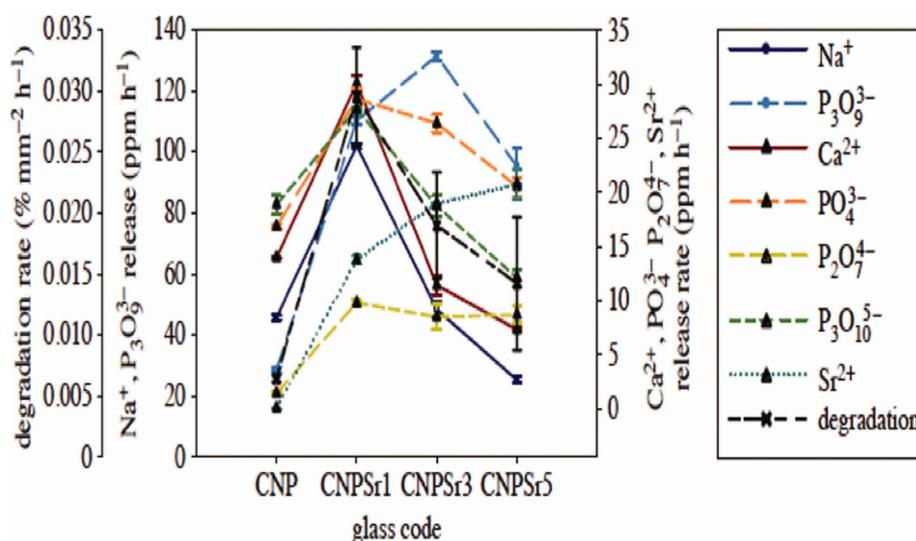
FIGURE 7. Degradation rate and ion release as a function of composition by Abou Neel et al.<sup>131</sup> [Color figure can be viewed in the online issue, which is available at [wileyonlinelibrary.com](http://wileyonlinelibrary.com).]
