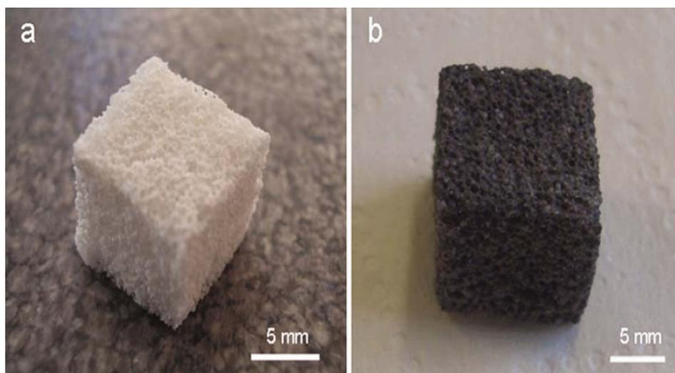
**FIGURE 6.** (a) GC-CEL2 scaffold and (b) GC-ICEL2 scaffold.<sup>130</sup> [Color figure can be viewed in the online issue, which is available at [wileyonlinelibrary.com](http://wileyonlinelibrary.com).]
