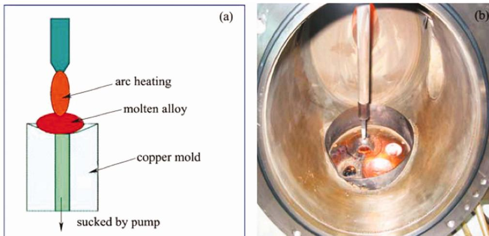
**FIGURE 10.** (a) schematic of casting and (b) set-up of soak mold casting.<sup>163</sup> [Color figure can be viewed in the online issue, which is available at [wileyonlinelibrary.com](http://wileyonlinelibrary.com).]
