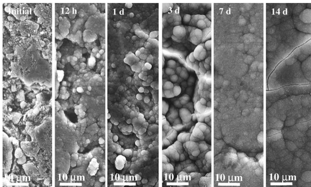
FIGURE 12. Scanning micrographs of the G-OHAp/700°C surface before and after soaking in SBF for different time periods.<sup>183</sup>
