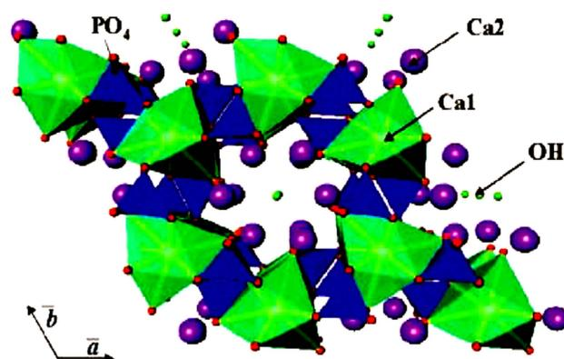
**FIGURE 11.** Proposed structure of hydroxyapatite.<sup>179</sup> [Color figure can be viewed in the online issue, which is available at [wileyonlinelibrary.com](http://wileyonlinelibrary.com).]
