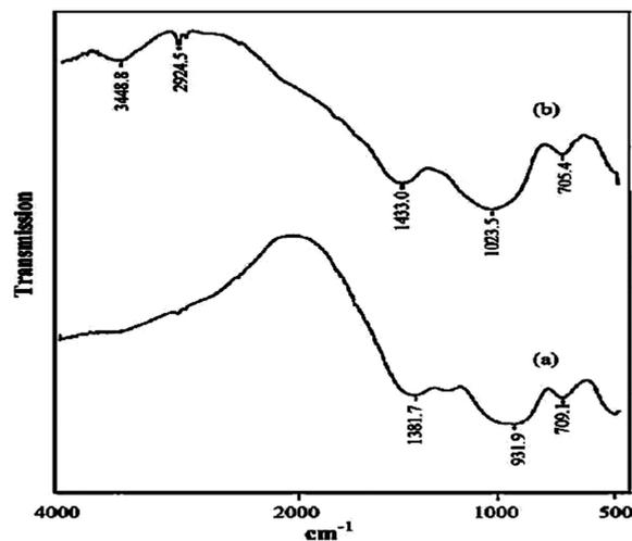
FIGURE 14. FT-IR spectra showing changes in GY glass after (a) 0 hr dipping and (b) 600 hr dipping in SBF solution.<sup>135</sup>
