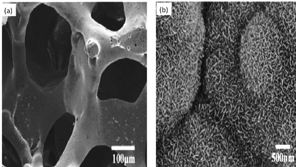
FIGURE 5. (a) 13-93 glass scaffold (b) formation of hydroxyapatite needles on the surface of 13-93 glass after 6 days in SBF.<sup>95</sup>
