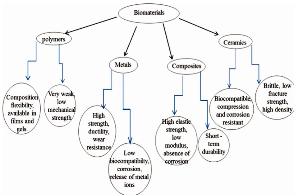
**FIGURE 1.** Schematic of classification of biomaterials. [Color figure can be viewed in the online issue, which is available at [wileyonlinelibrary.com](http://wileyonlinelibrary.com).]
