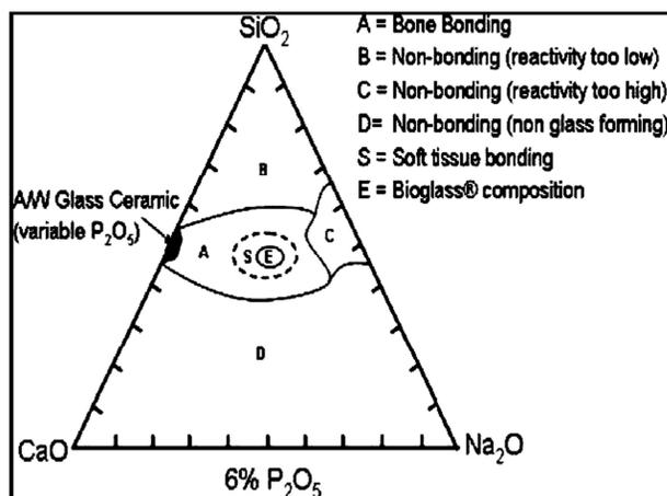
**FIGURE 2.** Ternary compositional diagram given for 45%  $\text{SiO}_2$ -24.5%  $\text{Na}_2\text{O}$ -24.5%  $\text{CaO}$ -6%  $\text{P}_2\text{O}_5$  glass by Hench for bone-bonding.<sup>13</sup>
