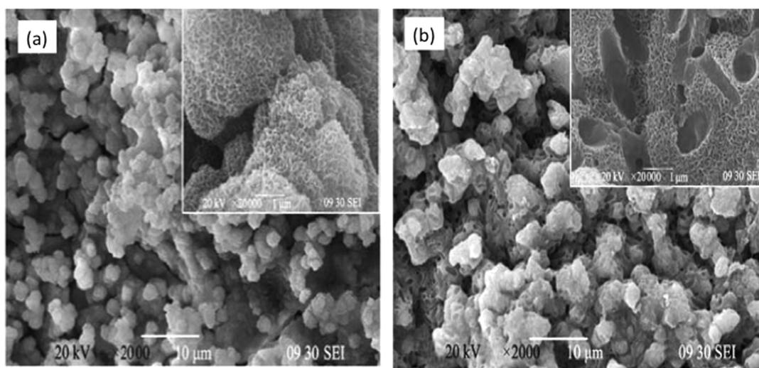
FIGURE 9. SEM images of MAO-treated  $Zr_{60.5}Cu_{19.5}Fe_5Al_{9.5}Ti_{5.5}$  BMG after immersion in SBF for (a) 5 and (b) 10 days.<sup>163</sup>
