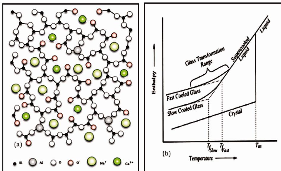
**FIGURE 3.** (a) Structure of glass and (b) enthalpy–temperature diagram.<sup>90</sup> [Color figure can be viewed in the online issue, which is available at [wileyonlinelibrary.com](http://wileyonlinelibrary.com).]
