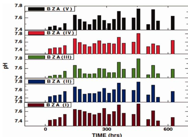
FIGURE 13. pH variation of glass dipped in SBF with time.<sup>71</sup> [Color figure can be viewed in the online issue, which is available at [wileyonlinelibrary.com](http://wileyonlinelibrary.com).]
