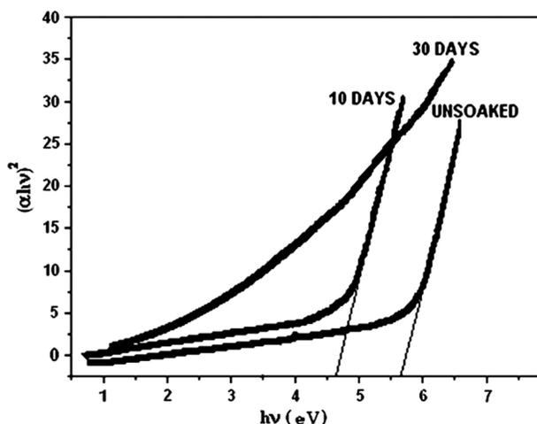
**FIGURE 15.** Change in band-gap of BZA glass after and before dipping in SBF solution.<sup>71</sup>
