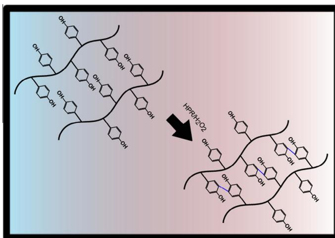
Fig. 5. Schematic mechanism of enzymatic reaction with horseradish peroxidase and hydrogen peroxide as catalyst system.
