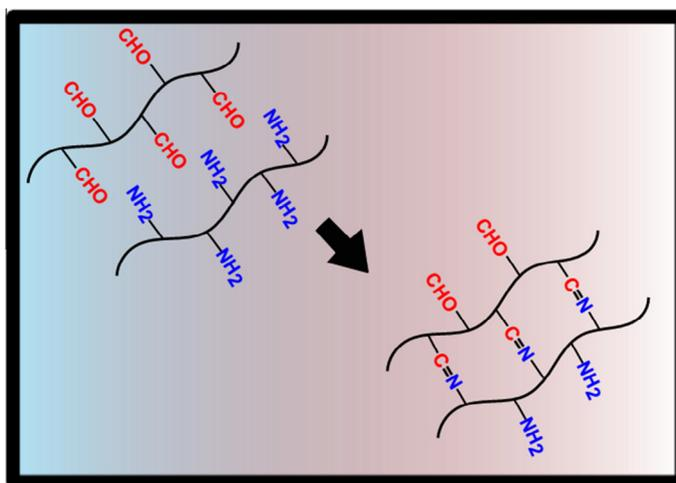
Fig. 4. Schematic mechanism of Schiff's base reaction between aldehyde and amine groups.
