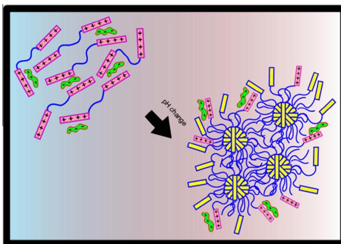
Fig. 7. Schematic mechanism of gelation driven by pH-inducing protonation–deprotonation transition of cationic hydrogel.
