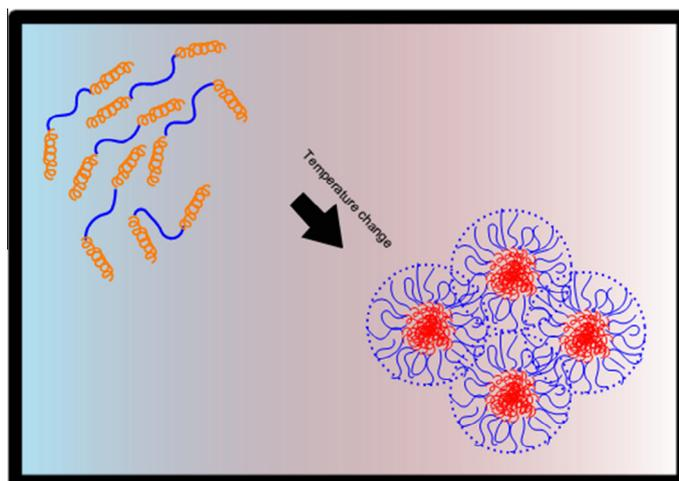
Fig. 6. Schematic mechanism of gelation driven by shifting of hydrophobic interaction under the change of temperature.
