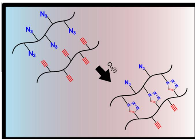
Fig. 2. Schematic mechanism of gelation by alkyne-azide click reaction with Cu(I) as catalyst.
