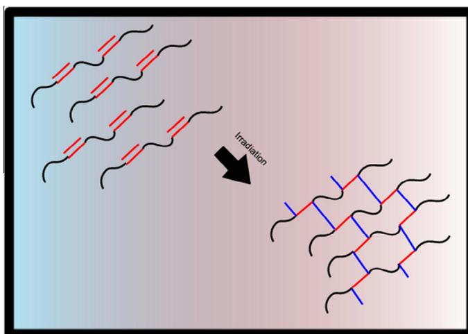
Fig. 1. Schematic mechanism of gelation by photocross-linking reaction of vinyl groups bearing polymers.
